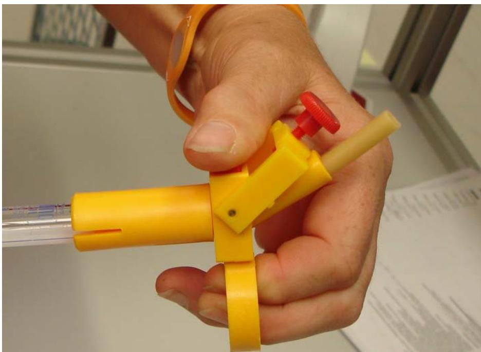
2) Push the shackle down and depress the push button all the way to take the spring pressure off the latex hose.
